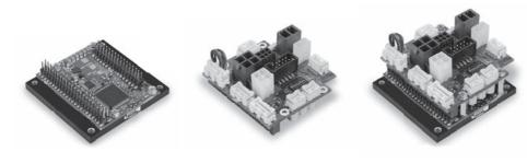
EPOS4 is a modular digital positioning controller. It is suitable for permanent magnet-activated DC motors and brushless, electronically commutated EC motors with incremental or absolute encoders with an operational range of up to 750 W continuous power. The variety of operating modes provides high flexibility: The controllers are suitable for use in a wide range of drive systems in automation and mechatronics.
