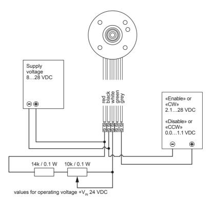
Figure 5 Set point «Set value speed» via external potentiometer and (depending on version) activation «Enable» or direction preselection «Direction» from external power supply
