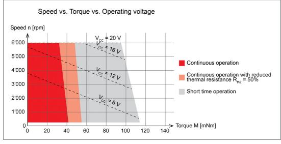
Figure 1 Speed / Torque / Operating voltage diagram
