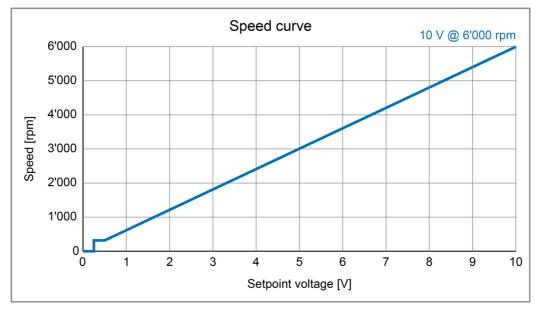
Figure 8 Speed as function of set value voltage
