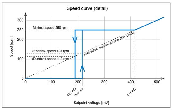
Figure 9 Speed as function of set value voltage – «Enable»
